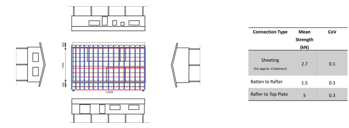
Failure when the load >strength: Failure Modes– Roof cladding: Batten-Rafter: Rafter-top plate:
