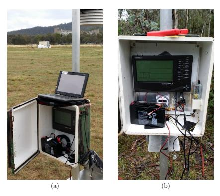
Figure 3.2: Data download using (a) Weatherlink  $(\mbox{\sc b})$  , and (b) the Raspberry Pi  $(\mbox{\sc b})$  system. Photographs taken by author.
