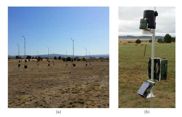
Figure 3.1: Davis Vantage Pro 2 Portable Automatic Weather Stations during the calibration phase; (a) set up at the UNSW Canberra Field Site, and (b) sensor array and console box. Photographs taken by author.
