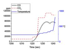
**Figure 2:** Temporal CO,  $CO_2$  and temperature profile during the transition from no ignition to flaming combustion. Radiant heating flux = 11.2 kW/m<sup>2</sup>). Air flow rate = 7.0 grams/min.
