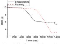
Figure 3: Mass loss profile for smouldering and flaming combustion. Initial mass: 10 grams.
