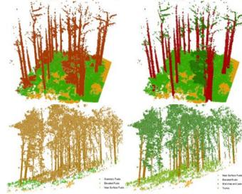
Fig. 3. Fuel strata classification comparison between the conventional (left) and the GIS-based methods (right) using Zebedee (top) and Riegl (bottom) terrestrial LiDAR systems.
