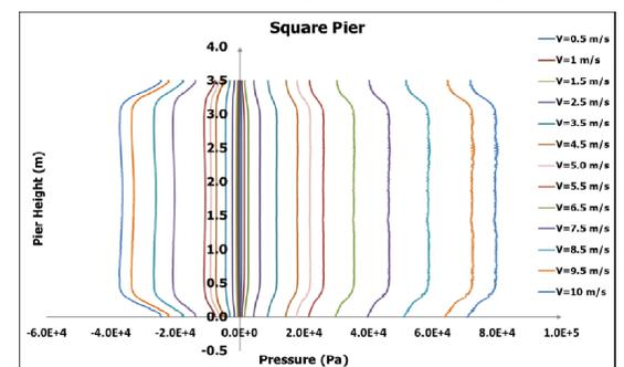
Fig2: Pressure distribution along the square pier height
