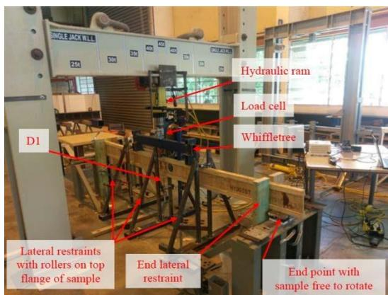
(C) ENGINEERED TIMBER JOISTS
