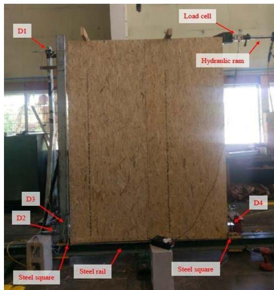
(B) MANUFACTURED SHEET WALL BRACING
