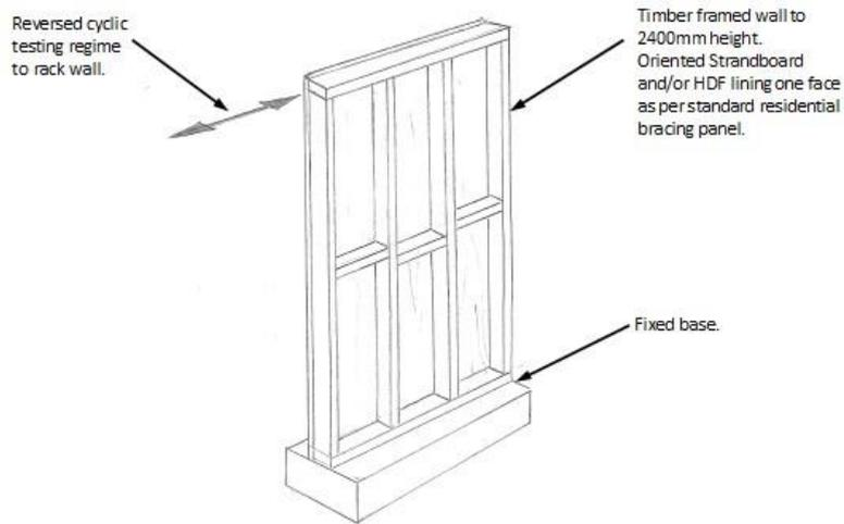
(B) MANUFACTURED SHEET WALL BRACING
