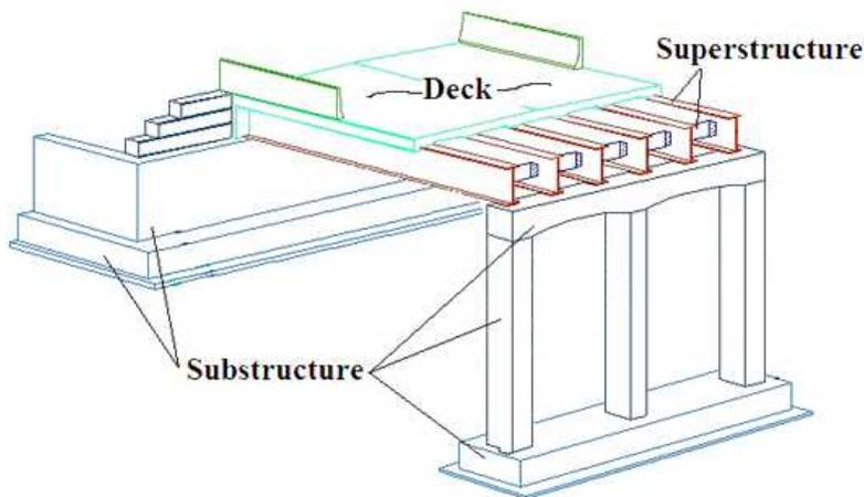
FIGURE 2: BRIDGE MAIN COMPONENTS (MDOT 2015)
