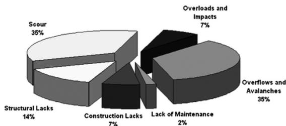
FIGURE 13: CAUSES OF BRIDGE COLLAPSE IN COLOMBIA[33]
