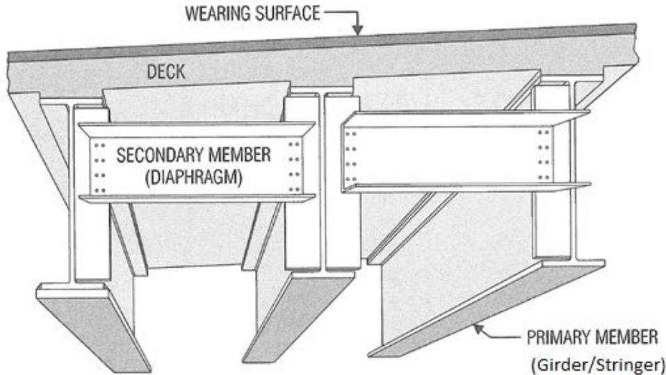
FIGURE 3: BRIDGE TYPICAL SUPERSTRUCTURE COMPONENTS [1]
