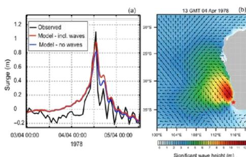
Figure 2. Simulated water levels for Cyclone Alby 1978 at Busseton (a) and associated wave heights (b) from coupled wave-surge model.
