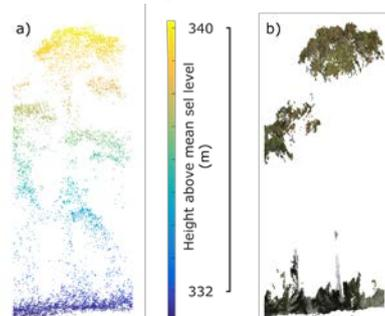
Figure 2. Laser scanning and SfM data captured from a UAS platform.
