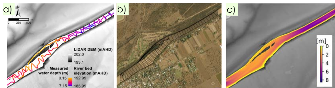
Figure 5 – Balonne River near St. George: a) measured bathymetric data; b) conformal map; c) reconstructed river bathymetry using conformal mapping.
