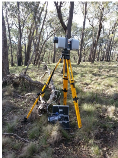
Figure 3.5 TLS setup in the field.
