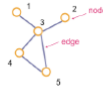
Fig. 1 Example of a graph with five nodes and five edges.
