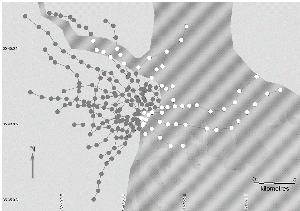
Figure 3.5: Graphical representation of the Tokyo Subway. The hypothetical inundation hazard footprint ( http://flood.firetree.net/ ) is indicated by the grey area ■ and the network components that coincide with the footprint are highlighted in white ○.
