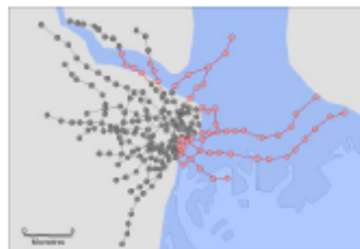
Fig. 2 Graph representation of the Tokyo Subway. Hypothetical inundation hazard footprint is indicated in blue and network components that coincide with the footprint are highlighted in red.
