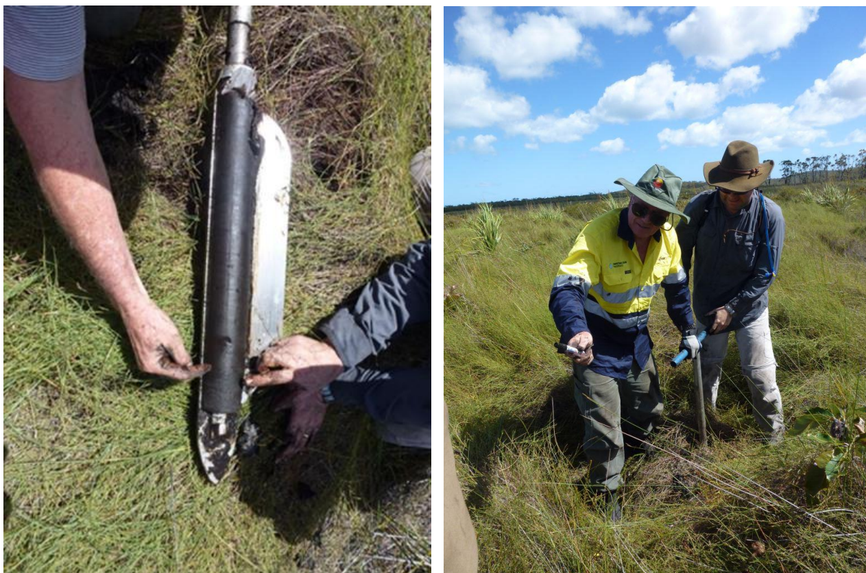
Figure 4.5. D-section (Russian) peat corer with core taken at Moon Point patterned fen in November 2013.
