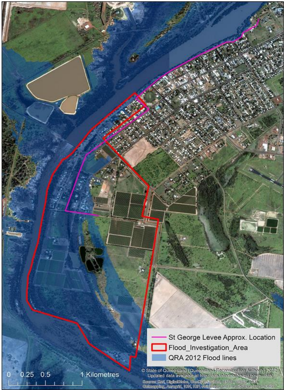
Figure 11: The approximate location of the levee (Source: Risk Frontiers, Data from Balonne Shire Council, 2013a, Balonne Shire Council, 2013b, Queensland Reconstruction Authority, 2012) Homes that will be outside the levee and unprotected, as well as inside the flood investigation area, are offered the three risk mitigation options.
