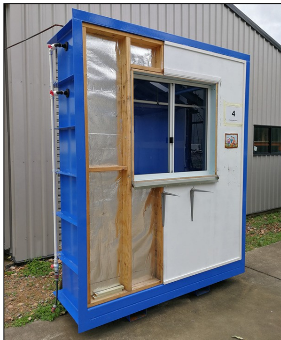
FIGURE 1. WDRS WITH WALL AND WINDOW TEST SAMPLE
