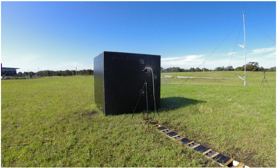
FIGURE 4.7: Photograph of the experimental setup for case D. Ground collectors are visible in the foreground (set in a frame and separated by sections of black plastic sheet).
