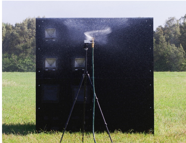
FIGURE 4.12: Photograph from Experiment A1, showing the concentrated ‘swirl’ of droplets emitted by the butterfly sprinkler.
