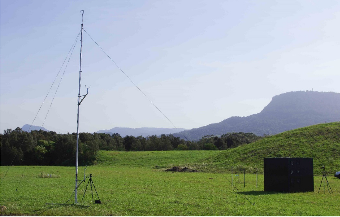
FIGURE 4.4: Photograph of the experimental setup, showing the meteorological mast near the cube. Three-axis ultrasonic anemometers were fitted at heights of 2 m and 10 m on the mast, and a two-axis ultrasonic anemometer was fitted at a height of 6 m.
