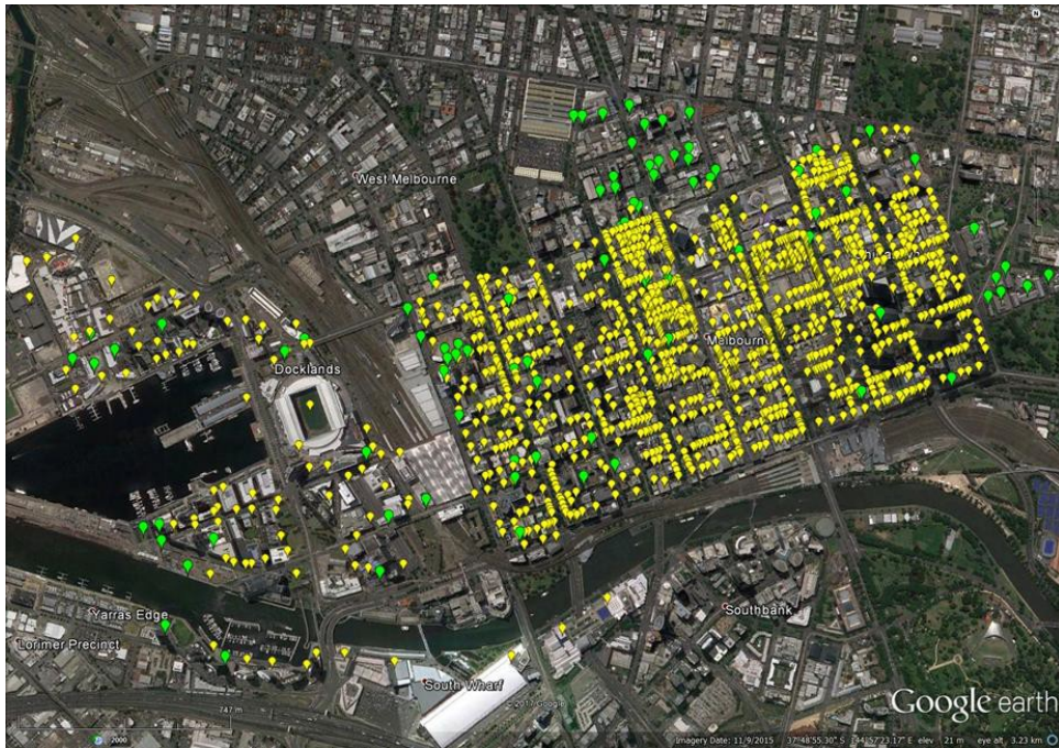
Figure 4: Buildings surveys in the Melbourne central business district with the capture of engineering parameters to enable mapping of earthquake vulnerability.
