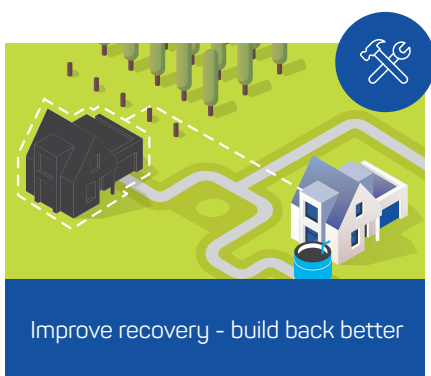
Figure 7: Property owners could reduce risk by making changes to road networks for response access, reducing exposure to hazards by relocating further from a managed vegetation area and improving resistance with provision of on-site water storage.
