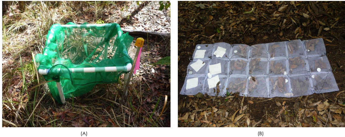
FIGURE 5: PHOTOS OF ASSEMBLED LITTERFALL TRAP (A) AND DECOMPOSITION BAG (B). EACH WAS LEFT AT THE SITE FOR ROUGHLY ONE YEAR TO MEASURE ANNUAL INPUT AND OUTPUT RATES OF FINE FUELS. 2
