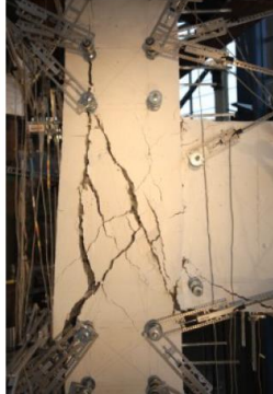
Instantly before axial failure
