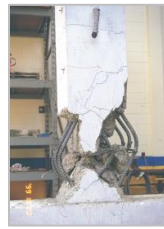
After axial load failure
