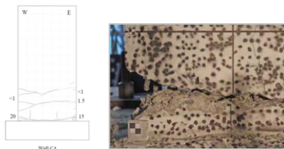
Figure 5-17: Comparison of simulated and experimental response of lightly reinforced walls for which a single crack is predicted, and a brief description of the observed failure mechanism
