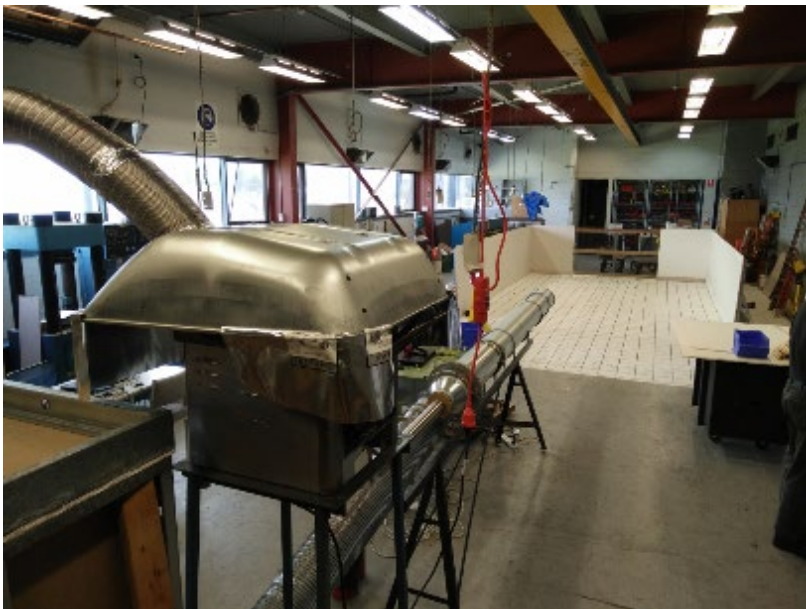
FIGURE 1: FIREBRAND DRAGON CONSTRUCTED AT OUR FACILITY TO GENERATE REPEATABLE UNIFORM FIREBRAND SHOWERS.
