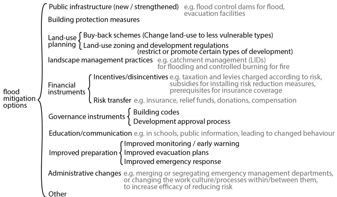
Fig. 3. A taxonomy of options that can be used for managing flood risk, showing the diversity of options available for consideration, as shown in part f of fig. 1 of the proposed framework. Although shown here for flood management, the general categories are applicable to other natural hazards as well. To obtain the best possible management outcomes, all of these options need to be considered jointly.
