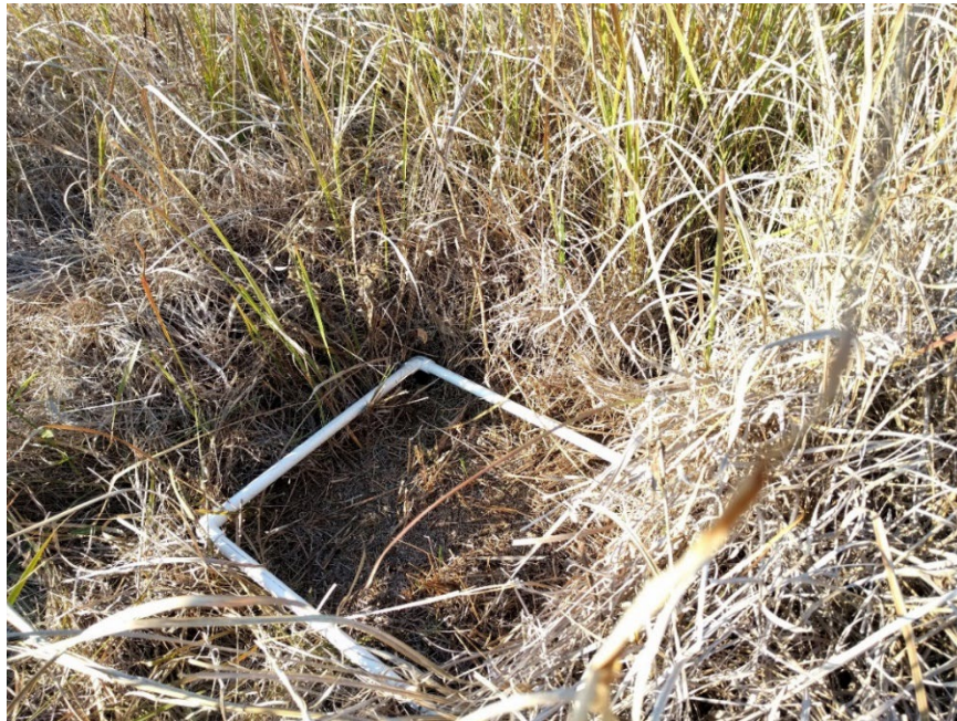
Figure A3. Example of application fuel sample quadrat to estimate grassland fuel load.
