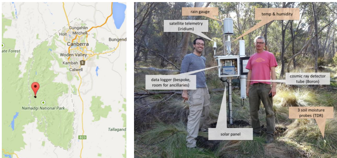
FIGURE 14. (LEFT) LOCATION OF THE NAMADGI COSMOZ STATION, AND (RIGHT) THE STATION COMPONENTS.
