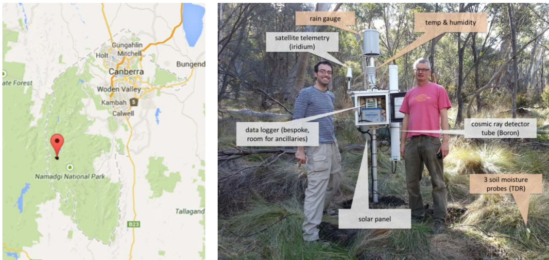
FIGURE 7. (LEFT) LOCATION OF THE NAMADGI COSMOZ STATION, AND (RIGHT) THE STATION COMPONENTS.
