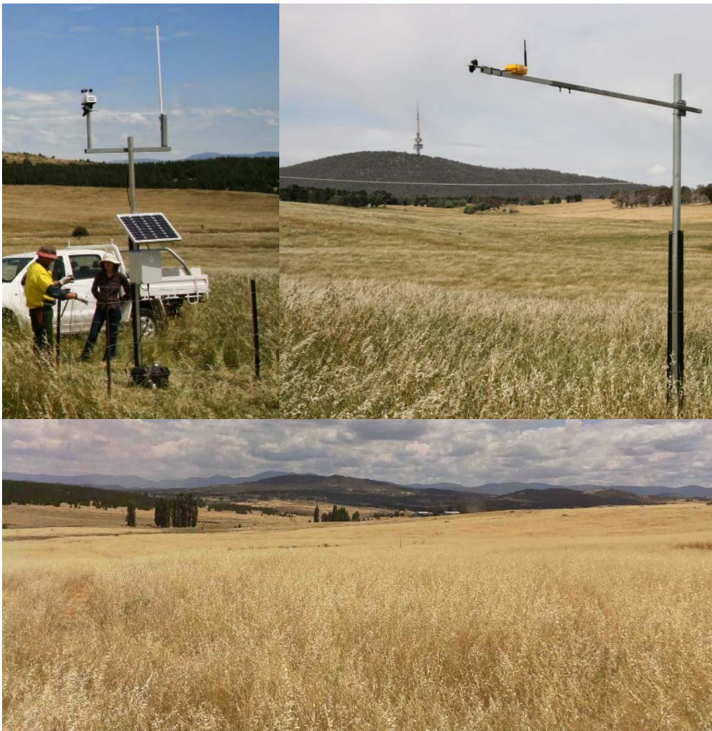
FIGURE 6. IN-SITU SENSORS FOR MONITORING GRASS CURING AND FUEL MOISTURE CONTENT. (TOP LEFT) METEOROLOGICAL STATION; (TOP RIGHT) ONE OF THE 5 SENSOR LOCATED ON THE SITE AND (BOTTOM) VIEW FROM THE RASBERRY PI CAMARA.
