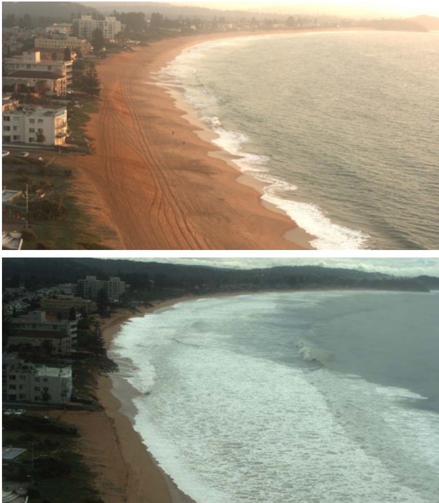
FIGURE 3: COMPARISON OF NARRABEEN'S COASTLINE PRIOR AND POST TO THE SEVERE STORM IN APRIL 2015. THE SHORELINE RETREAT IS MEASURED AT 25 METRES. (PHOTO: DR MITCHEL HARLEY)
