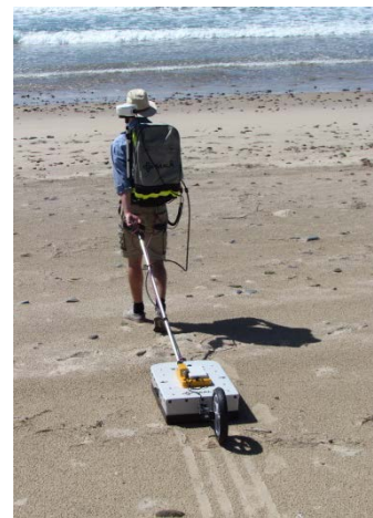
FIGURE 1: FIELD INVESTIGATIONS TEAM CONDUCTING THE GPR SURVEY AT OLD BAR IN MARCH 2015. LEFT-HAND IMAGE: ANDREW MCPHERSON AND SCOTT NICHOL, RIGHT-HAND IMAGE: FLOYD HOWARD.
