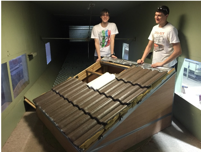
FIGURE 8. UNDERGRADUATE STUDENTS AT JAMES COOK UNIVERSITY CONTRIBUTE TO THE PROJECT BY CONDUCTING WIND LOAD CHARACTERIZATION TESTING FOR ROOFING TILES IN THE CTS WIND TUNNEL AS PART OF A FOURTH YEAR THESIS PROJECT
