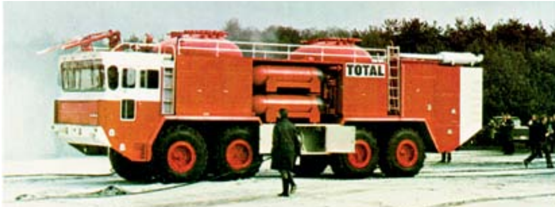
A late twentieth century 12,000 kg dry chemical fire truck.
