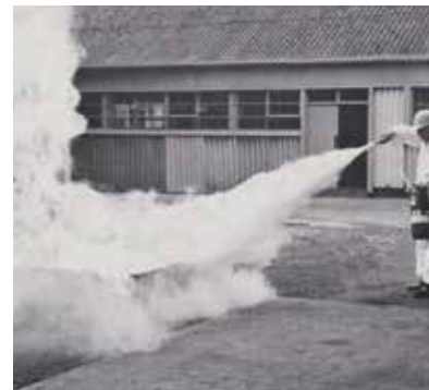
A stored pressure dry chemical extinguisher in action.
