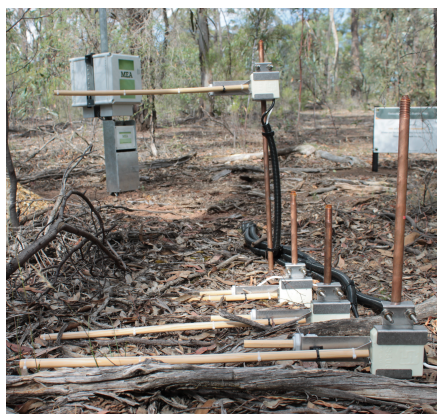
Fig. 1 Typical Array of four Fuel Moisture Sticks attached to a logger and modem.
