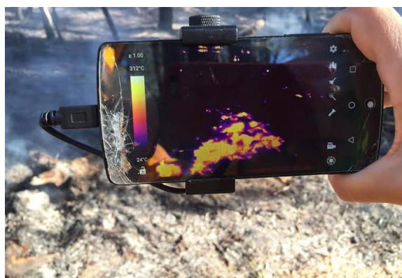
FIGURE 3. TESTING THE THERMAL MICROBOLOMETER (THERM-APP) IN HAND AT THE CHRISTMAS HILLS FIRESCAPE BURN.
