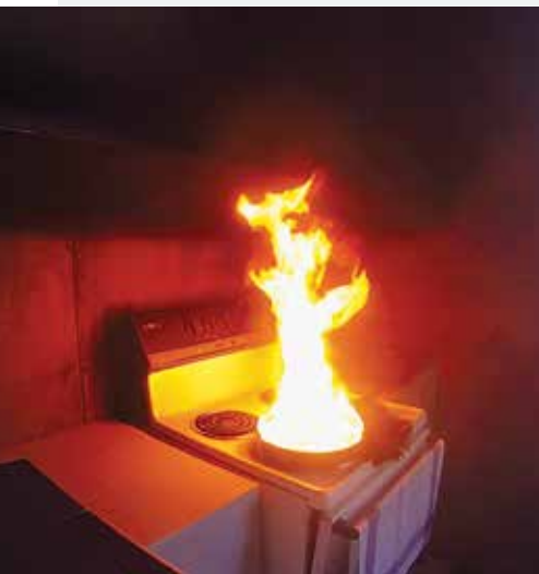
FRNSW Fire Investigation and Research Unit conducted test smoke alarm burns at the FRNSW Research and Training Facility in Londonderry, NSW.
