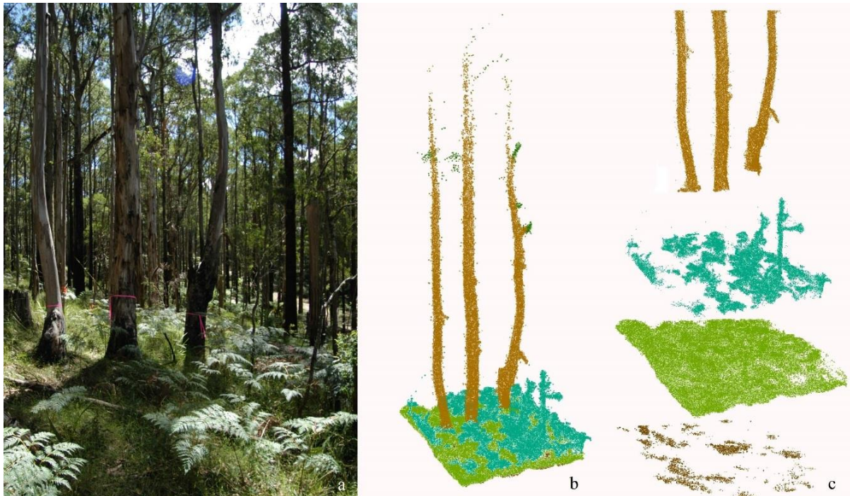
Figure 5. TLS-derived fuel structural classification compared with a photograph taken at Plot 2. 5a. A photograph of forest fuel; 5b. An overview of LiDAR derived fuel strata; 5c. The classified fuel strata from top to bottom, including tree trunks, elevated fuel, near surface fuel, and surface fuel.
