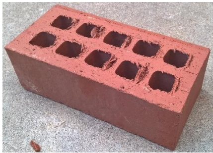
(a) Perforated clay brick (b) 3 mm thick wall ties; inset shows the bent shape as used in walls Figure 2: Standard masonry units and wall ties
