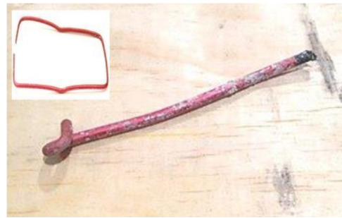
(a) Perforated clay brick (b) 3 mm thick wall ties; inset shows the bent shape as used in walls Figure 2: Standard masonry units and wall ties
