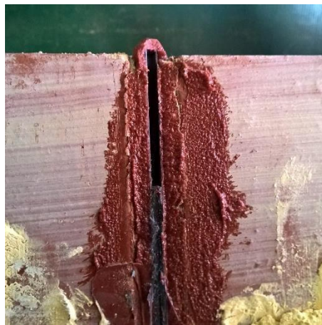
(b) Slip of the FRP reinforcement associated with IC debonding formation
