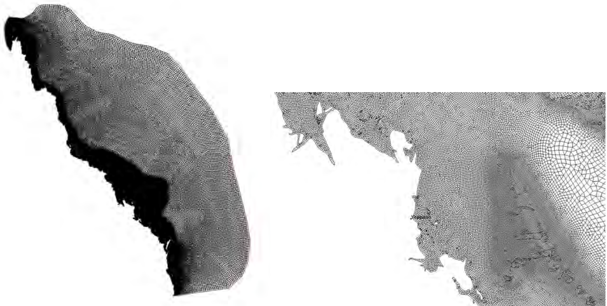
Figure 10. Flexible finite volume triangular mesh used for storm tide modelling in the Coral Sea.
