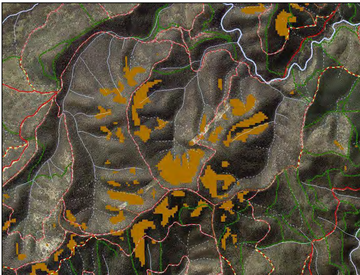
FIGURE 4 - POTENTIAL SOURCES OF DEBRIS FLOW WITHIN THE WOMBAT CREEK BURN; EROSION SOURCE AREAS ARE INDICATED BY BROWN SHADING
