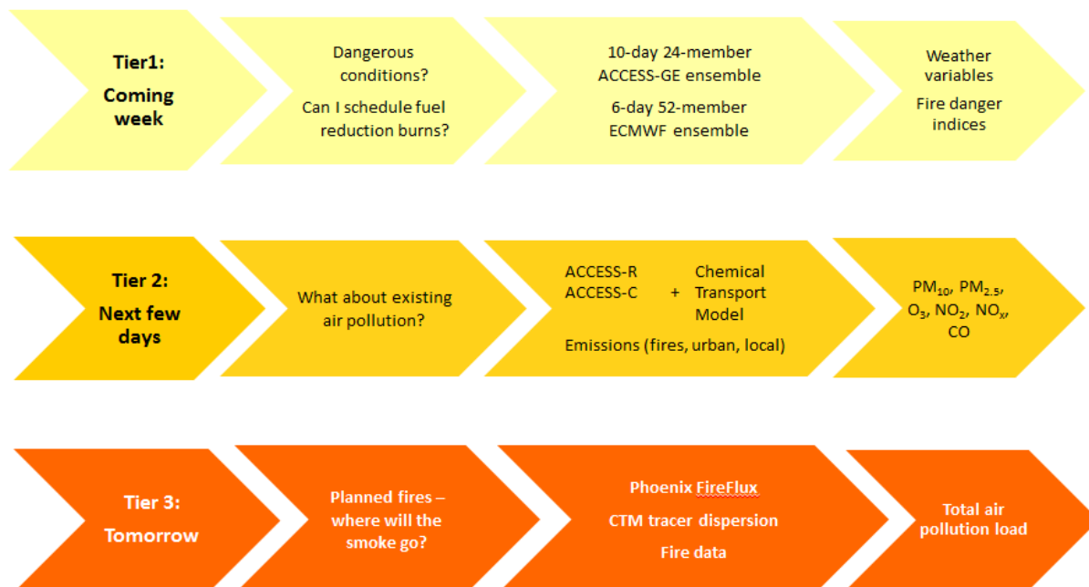
FIGURE 1. 3-TIERED SMOKE FORECASTING SYSTEM
