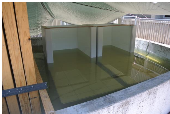
FIGURE 38: TWO SAMPLES IN THE WATER TANK DURING THE FLOOD SIMULATION
