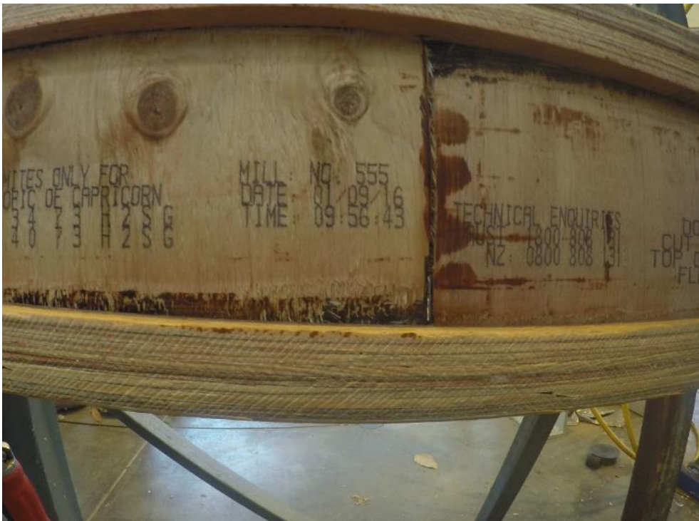
FIGURE C22: FAILURE OF H2 TREATED TIMBER T SECTIONS WET-WET SAMPLES: WEB DISLODGED FROM FLANGES
