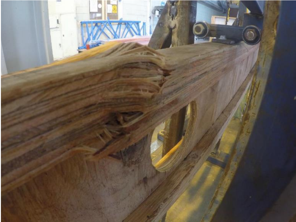
FIGURE C21: FAILURE OF H2 TREATED TIMBER T SECTIONS WET-WET SAMPLES: TOP FLANGE COLLAPSE (LOCALISED BUCKLING) AT LOADING POINTS
