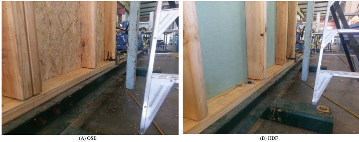
FIGURE B9: STUD WITHDRAWAL FROM BOTTOM PLATE
