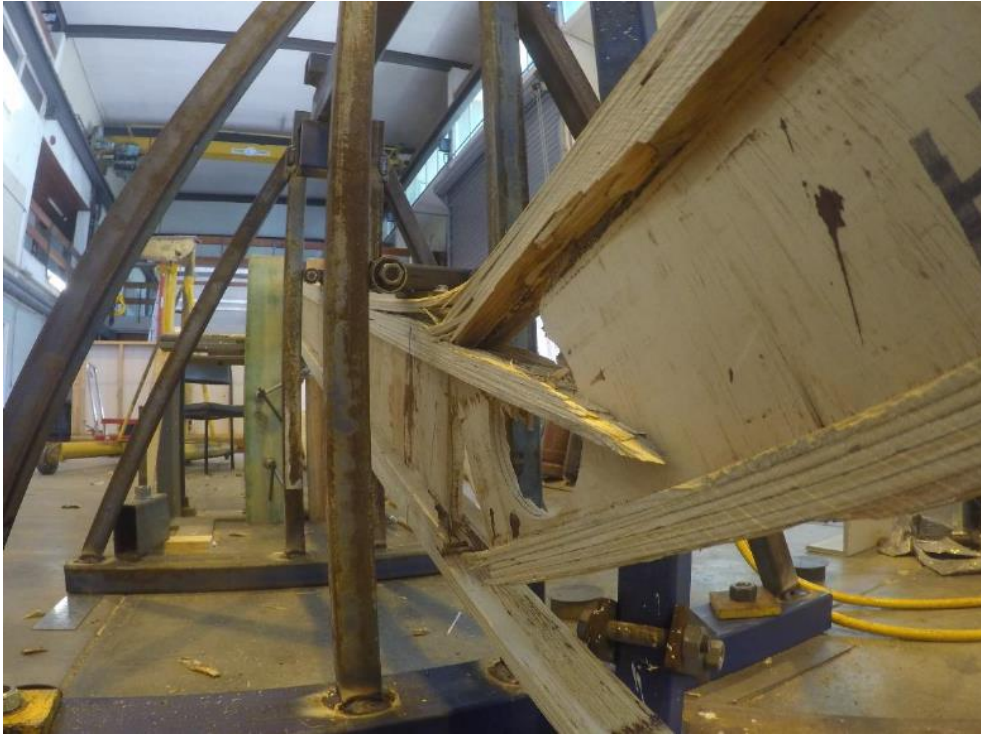
FIGURE C23: FAILURE OF UNTREATED TIMBER T SECTIONS DRY-DRY SAMPLES: TOP AND BOTTOM RUPTURE AND CRACKED WEB
