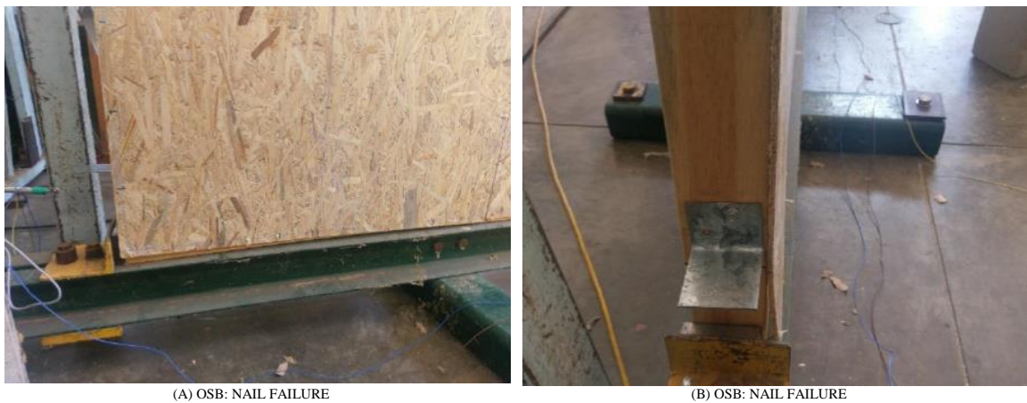
FIGURE B10: NAIL FAILURE (DRY-DRY SAMPLES)
