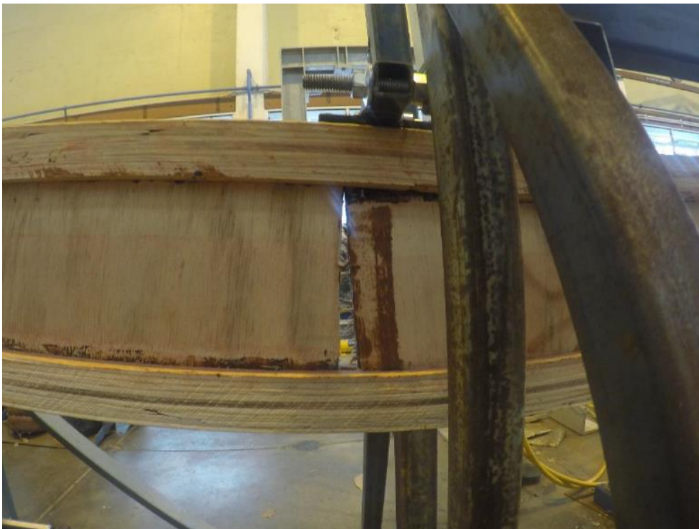
FIGURE C28: FAILURE OF UNTREATED TIMBER T SECTIONS WET-WET SAMPLES: TOP FLANG AND WEB COLLAPSE
