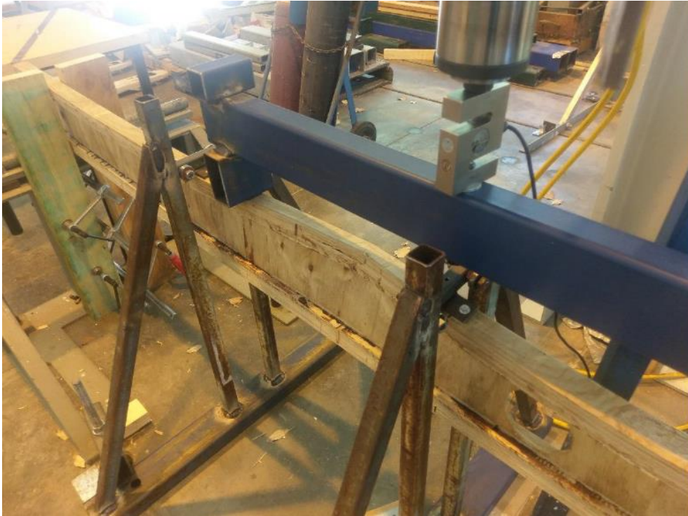
FIGURE C25: FAILURE OF UNTREATED TIMBER T SECTIONS WET-DRY SAMPLES: TOP FLANGE COLLAPSE (LOCALISED BUCKLING) AT LOADING POINTS
