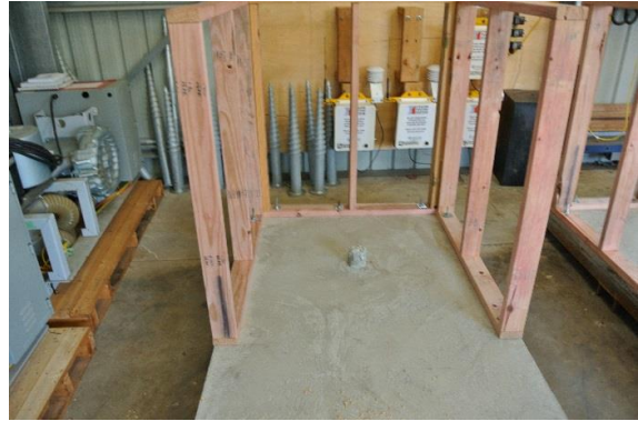
FIGURE 19: TWO LATERAL AND ONE END STUD WALLS
