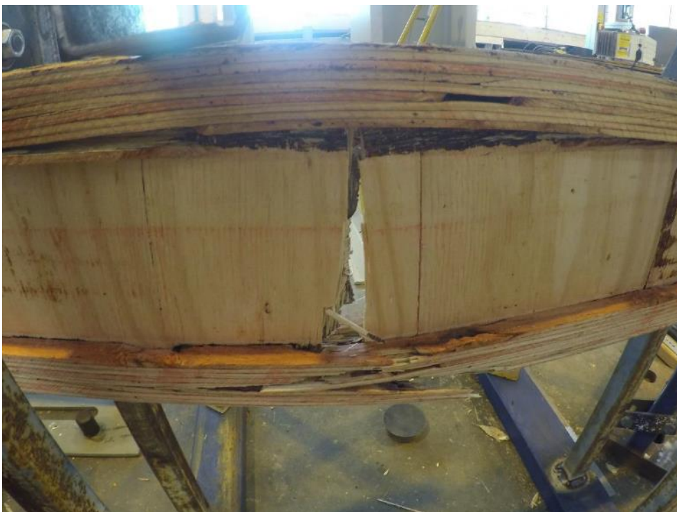
FIGURE C18: FAILURE OF H2 TREATED TIMBER T SECTIONS DRY-DRY SAMPLES: BOTTOM FLANGE RUPTURE AND WEB DISLODGED FROM FLANGES
