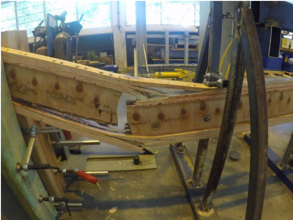
FIGURE C17: FAILURE OF H2 TREATED TIMBER T SECTIONS DRY-DRY SAMPLES: TOP AND BOTTOM RUPTURE AND CRACKED WEB
