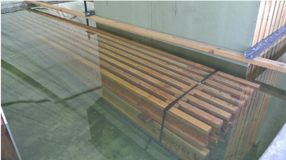
FIGURE 50: SAMPLES SUBMERGED IN THE IMMERSION TANK DURING THE FLOOD SIMULATION
