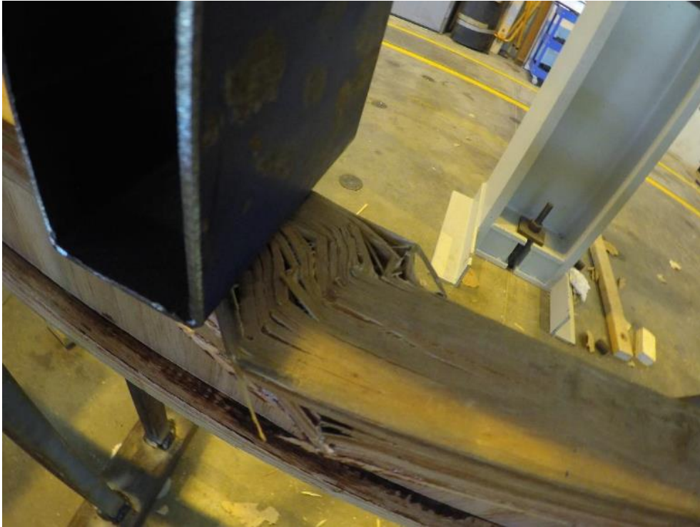
FIGURE C19: FAILURE OF H2 TREATED TIMBER T SECTIONS WET-DRY SAMPLES: TOP FLANGE COLLAPSE (LOCALISED BUCKLING) AT LOADING POINTS
