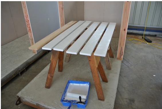
FIGURE 4: PINE PLANKS USED TO SIMULATE DOOR JAMBS
