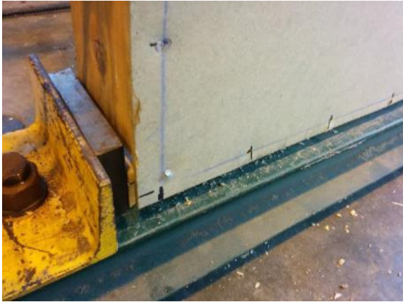
(A) HDF: NAIL FAILURE
