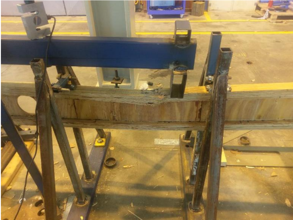
FIGURE C27: FAILURE OF UNTREATED TIMBER T SECTIONS WET-WET SAMPLES: TOP FLANGE COLLAPSE (LOCALISED BUCKLING) AT LOADING POINTS
