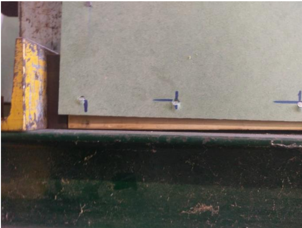
FIGURE B16: OSB BOTTOM PLATE FAILURE (DRY-DRY SAMPLES)
