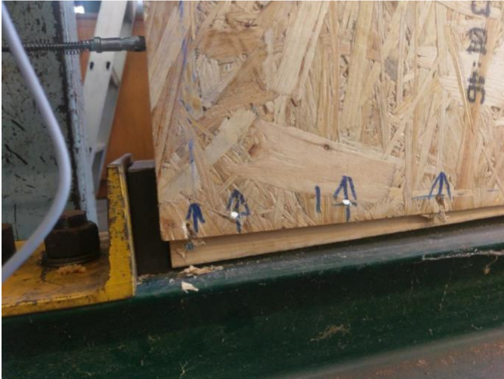
FIGURE B11: OSB BRACE SHEETING FAILURE (DRY-DRY SAMPLES)
