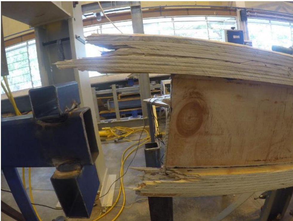
FIGURE C24: FAILURE OF UNTREATED TIMBER T SECTIONS DRY-DRY SAMPLES: TOP AND BOTTOM FLANGES CRACKED AT WEB JOINT
