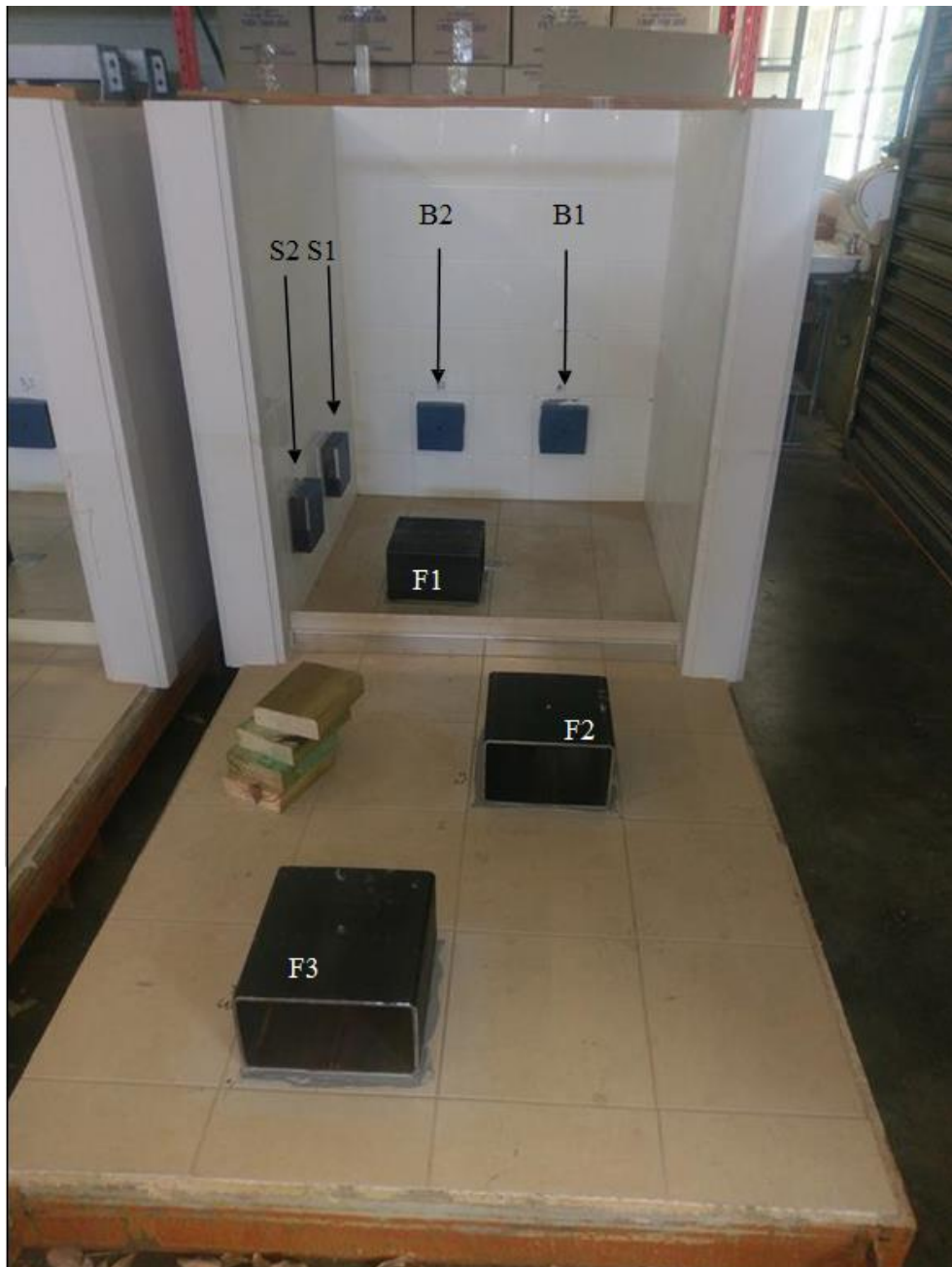
FIGURE 39: LOCATION OF TILES TO BE TESTED AND RHS ANCHORING POINTS BONDED ON TILES
