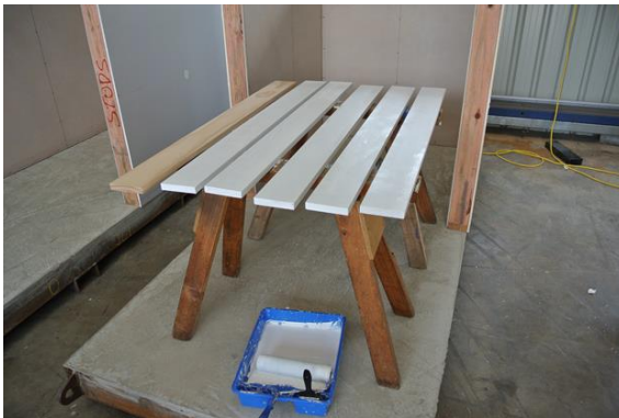
FIGURE 20: PINE PLANKS USED TO SIMULATE DOOR JAMBS
