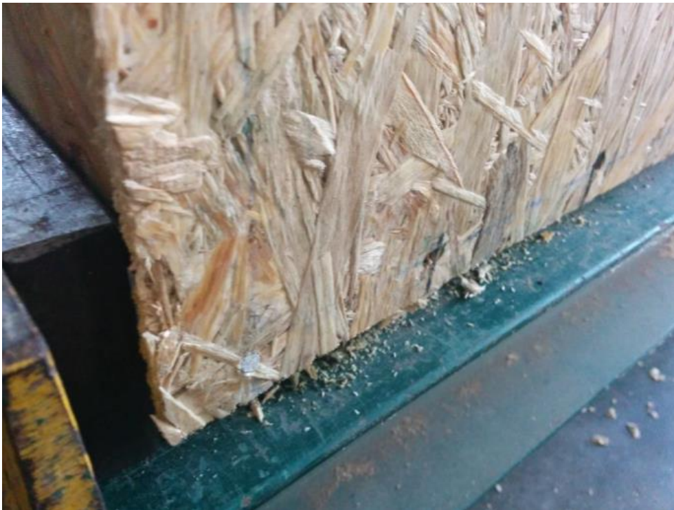
FIGURE B14: OSB BOTTOM PLATE FAILURE (DRY-DRY SAMPLES)
