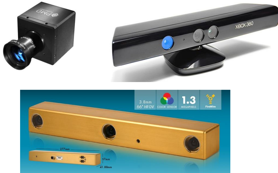
FIGURE 4 – EXAMPLES OF A) TOF (PMD CAMCUBE), B) STRUCTURED LIGHT (MICROSOFT KINECT) AND C) STEREO (POINTGREY BUMBLEBEE X3) CAMERA TECHNOLOGY.
