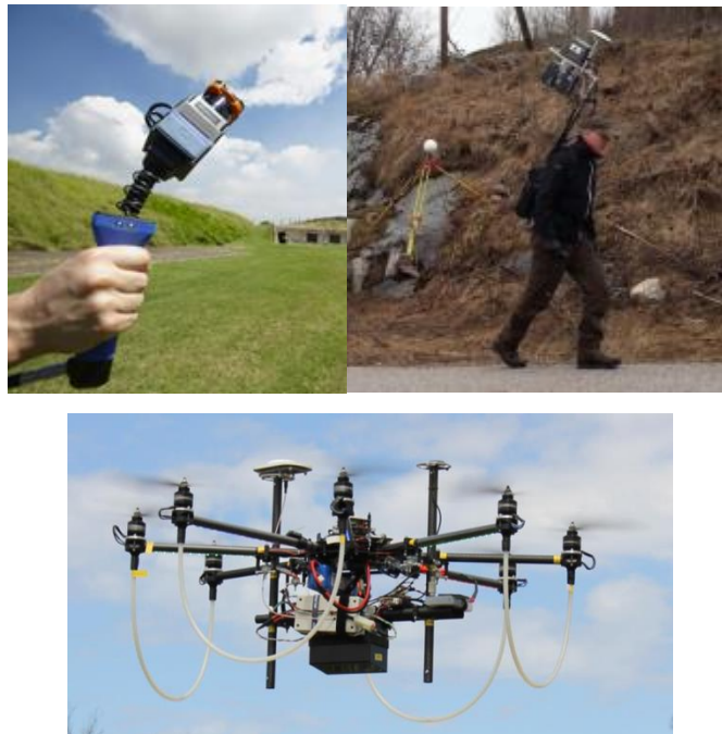
FIGURE 2 – THE ZEB1 LASER SCANNER, THE BACK PACK SCANNER USED IN LIANG ET AL. (2014) AND THE UAV LASER SCANNER DESCRIBED IN WALLACE ET AL. (2012)
