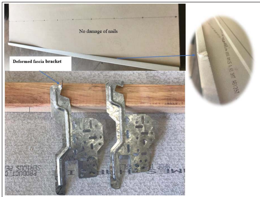
Figure 16: Failure mode for Test 3 – Photograph by Lalin Chhoeuk
