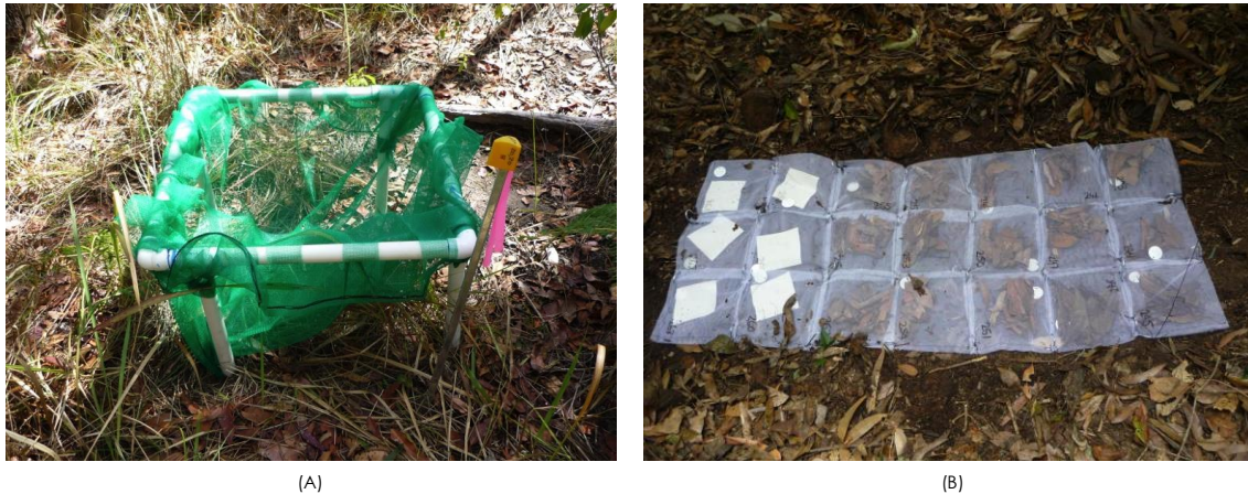
FIGURE 3: PHOTOS OF ASSEMBLED LITTERFALL TRAP (A) AND DECOMPOSITION BAG (B). EACH WAS LEFT AT THE SITE FOR ROUGHLY ONE YEAR TO MEASURE ANNUAL INPUT AND OUTPUT RATES OF FINE FUELS. 2
