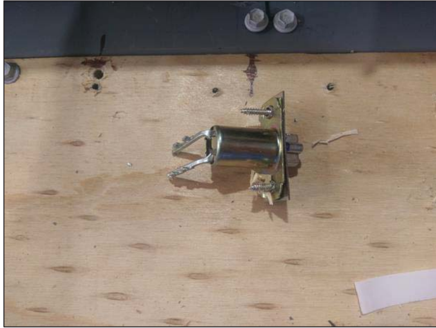
Figure 23: Trial SS5a Broken Lock Mechanism
