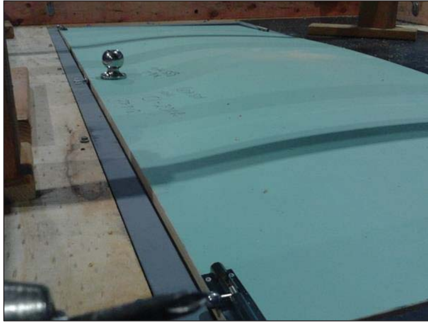
Figure 15: Trial SS4 Door Deflection during Test
