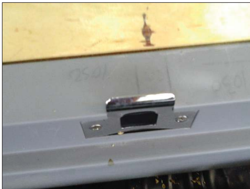
Figure 8: Trial SS2 Strike Plate Bent
