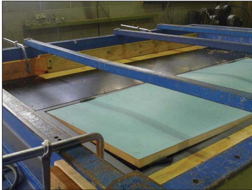
Figure 6: Trial SS2 door deflection during test
