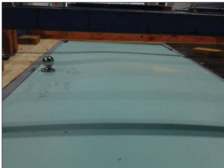
Figure 14: Trial SS4 Door Deflection during Test
