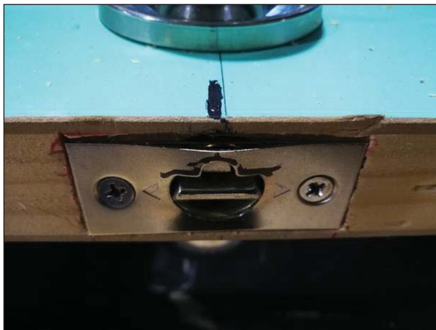
Figure 13: Trial SS4 Jammed Lock Mechanism
