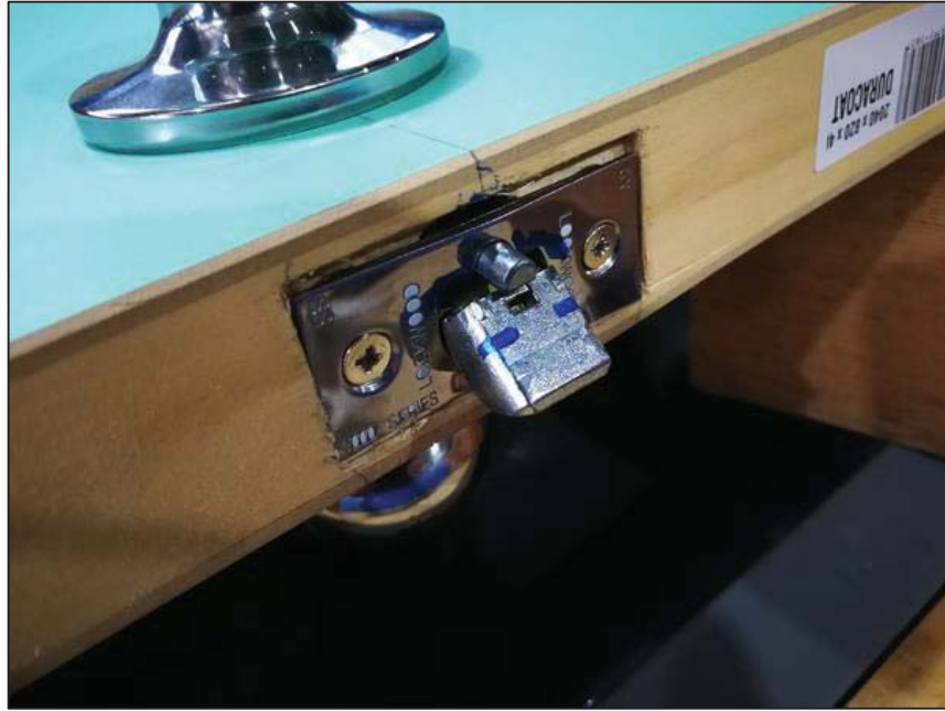
Figure 25: Trial SS6 Damage to Lock Mechanism
