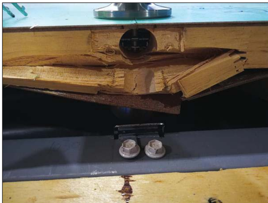
Figure 21: Trial SS5a Broken Lock Mechanism and Damaged Door
