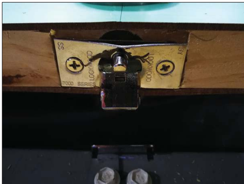
Figure 16: Trial SS5 Broken Lock Mechanism
