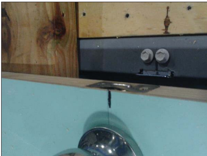
Figure 10: Trial SS3 Damaged Lock Mechanism
