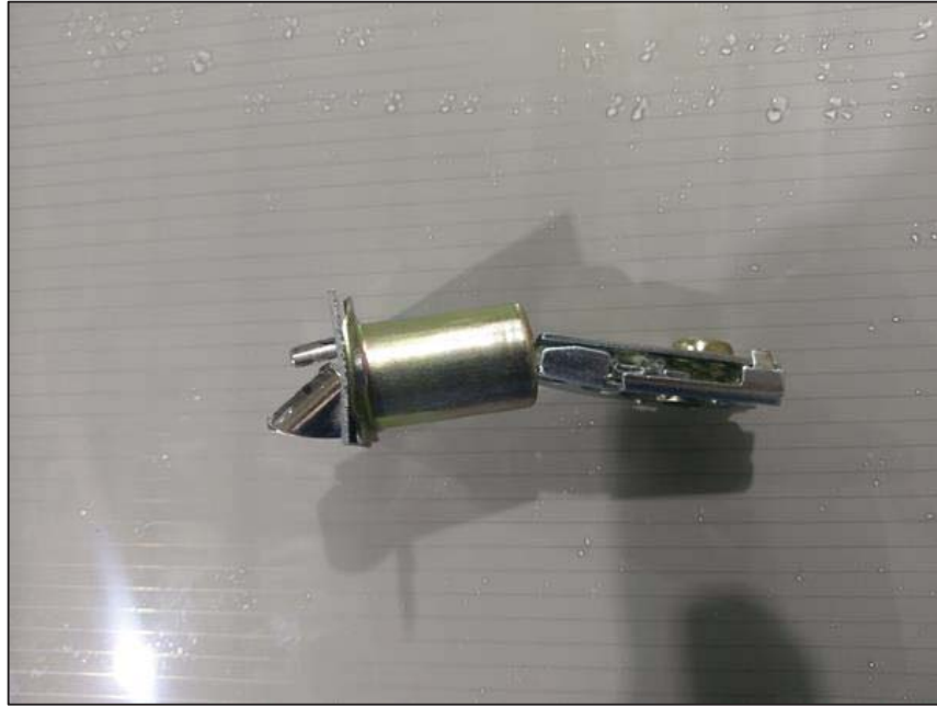
Figure 19: Trial SS5 Broken Lock Mechanism
